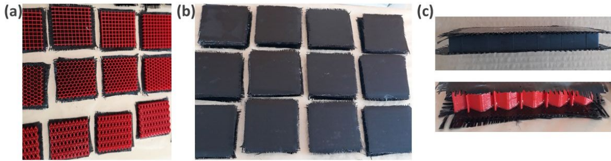
Figure 3. Production steps of sandwich composite specimens: (a) placement of carbon fabrics in the lower part of the core structure, (b) placement of carbon fabrics in the upper part of the core structure, and (c) sandwich composites produced.
